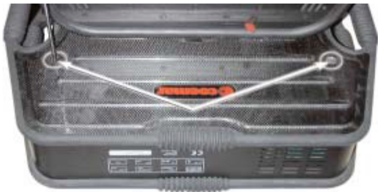
Figure W12/E Removing covers
